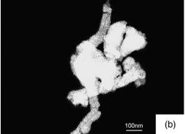
Fig. 1. TEM images of A-MWCNTs (a) and TiO<sub>2</sub>/MWCNTs composites (b).
