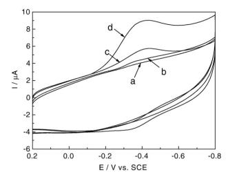
Fig. 7. CVs at 100 mV/s in pH 7.0 PBS for  $\text{TiO}_2/\text{MWCNTs}$  GC electrodes in PBS containing no  $\text{H}_2\text{O}_2$  (a), as (a) in the presence 0.2 mM of  $\text{H}_2\text{O}_2$  (b), (c) and (d) as (a) and (b) for Mb–TiO $_2/\text{MWCNTs}$  modified GC electrodes.
