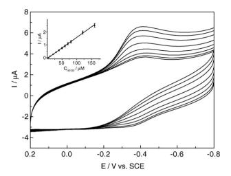
**Fig. 8.** CVs of Mb–TiO $_2$ /MWCNTs GC electrode in the presence different concentration of H $_2$ O $_2$  in PBS (pH 7.0) at 100 mV/s, from inner to outer 0, 4, 10, 20, 40, 80, 120 and 160  $\mu$ M. Inset: the catalytic response vs. hydrogen peroxide concentrations.
