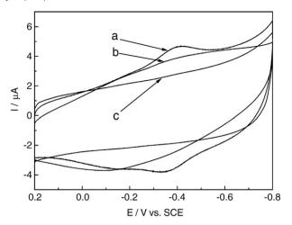
**Fig. 4.** CVs obtained with Mb–TiO $_2$ /MWCNTs film modified GC electrodes (a), TiO $_2$ /MWCNTs film modified GC electrodes (b) and bare GC electrodes (c) in 0.1 M PBS (pH 7.0) at 100 mV/s.
