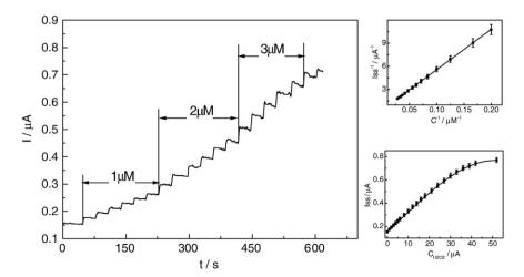
Fig. 9. Amperometric response of Mb-TiO<sub>2</sub>/MWCNTs GC electrode with successive addition of H<sub>2</sub>O<sub>2</sub> to the 0.1 M pH 7.0 PBS under stirring. The applied potential was -0.4 V.
