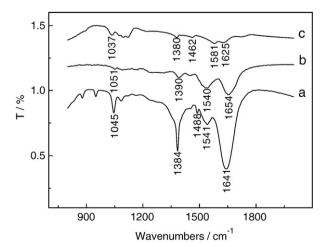
Fig. 3. FTIR spectra of Mb-TiO<sub>2</sub>/MWCNTs (a), free Mb (b), TiO<sub>2</sub>/MWCNTs (c) film.
