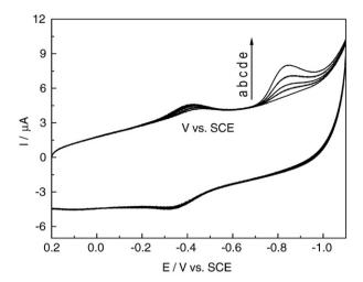
Fig. 10. CVs at 100 mV/s in pH 7.0 PBS for Mb– $\text{TiO}_2$ /MWCNTs modified GC electrode in PBS containing no NO (a), as (a) in the presence 0.1, 0.2, 0.4 and 0.8 mM of NO (b, c, d and d).
