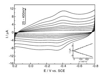
**Fig. 5.** CVs of Mb–TiO<sub>2</sub>/MWCNTs film modified GC electrodes in 0.1 M pH 7.0 PBS at different scan rates. The scan rate from inner to outer are 25, 50, 75, 100, 150, 200, 300, 400 mV/s respectively. Inset: plot of peak currents vs. scan rates.
