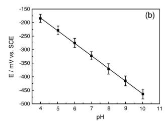
Fig. 6. (A) CVs of Mb–TiO<sub>2</sub>/MWCNTs film modified GC electrodes in 0.1 M PBS at various pH values: 5.0 (b), 7.0 (d), 9.0 (f) at scan rate of 100 mV/s. (B) Effect of pH on formal potential of Mb–TiO<sub>2</sub>/MWCNTs film modified GC electrodes in 0.1 M PBS.
