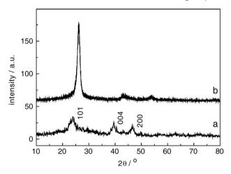
Fig. 2. XRD pattern of TiO<sub>2</sub>/MWCNTs (a), acid-treated MWCNTs (b).
